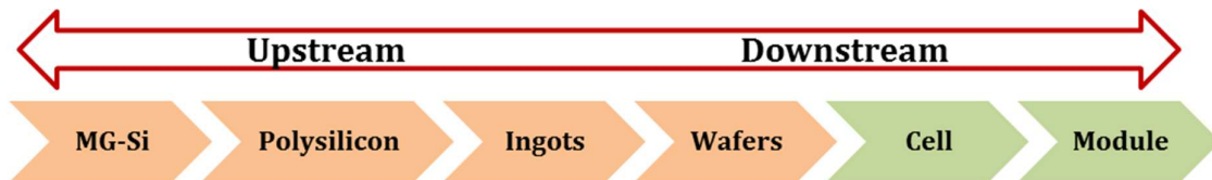
Figure 1: c-Si PV module supply chain
